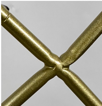
Shev's original back design chair welds
